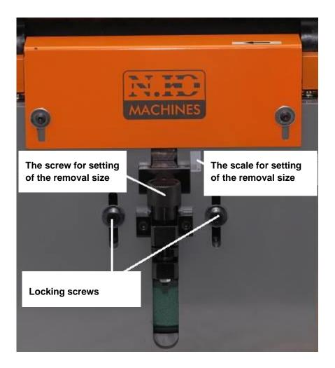
In case you need to use the maximum possible removal of the device, divide the required bevelling into several steps.
