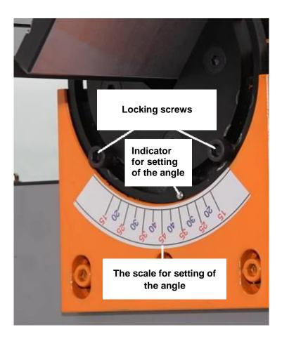
Loosen the screws on both sides. Tilt the prism to the desired angle and tighten the locking screws.
